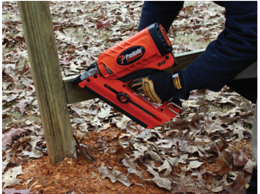
A cordless nailer like the Paslode model shown is an excellent time and labor saver for any major framing project.
